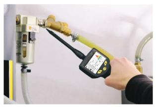
Leak detection with focus tube
