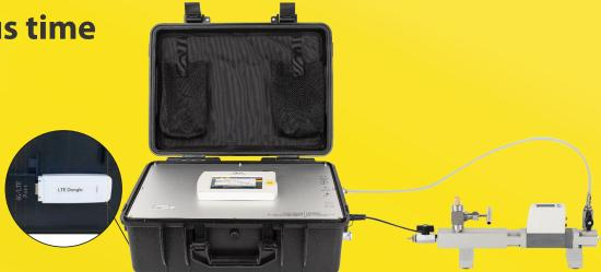
By connecting a LTE/4G modem to the designated USB port, S600 can be monitored remotely through S4A software
